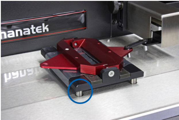
Sled is positioned on lift pins
