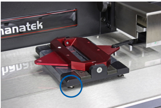
Lift pins retract into the instrument and the sled is placed in the same position each time
