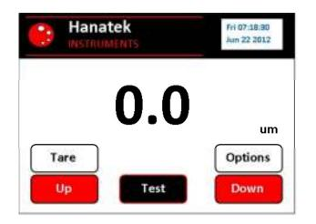
Push the "Down" button so the foot is in the DOWN position.
