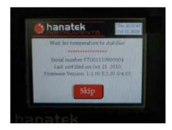
The instrument automatically switches into measurement mode when stability is reached (usually <2 mins).
