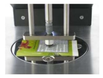
Press the down button to lower the measurement foot. Allow for the measurement to stabilise and record the reading displayed.
