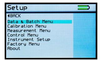
The Setup Screen is used to customise the instrument to the user's preference. Pressing the Up and Down buttons navigates through the options, pressing the Enter button selects that option.
