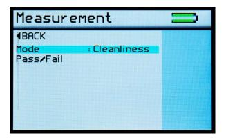
The Measurement Screen is used to configure the instruments measurement mode to the user's preference. Pressing the Up and Down buttons navigates through the options, pressing the Enter button selects that option.
