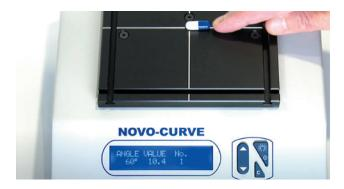
Simple checking of curved surfaces
