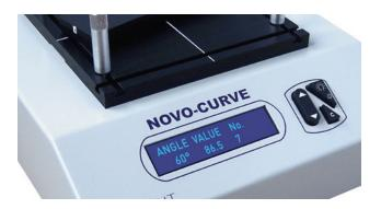
**Detailed analysis of results** USB data transfer of results to Novo-Soft for further analysis and export to CSV.
