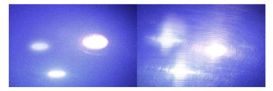
Haze is an important measure for highly polished metals and is often associated with polishing marks and machining direction.
