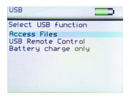
Access Files – Allows access to measurement and configuration files on the instrument. The instrument appears as a USB drive named NG-METER. When selected the display on the instrument shows a USB memory key as shown below –
