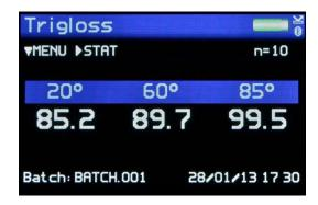
With the pass / fail feature enabled, the Novo-Gloss will compare each measurement angle to user defined tolerances, if the gloss reading is within specification the angle header will be displayed in green. If the reading falls outside the tolerances the header is marked in red.
