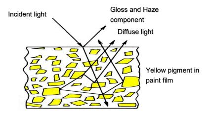
The Novo-Gloss compensates for reflection from within the coating for highly reflective pigments, metallic coatings and speciality pigments, allowing the haze of any painted surface to be measured.
