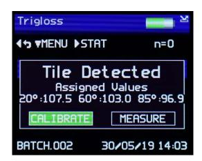
Two options are available: either to "Calibrate" the instrument on the calibration tile before making the measurement or to "Measure" without performing a calibration. Using the Left / Right (3) and Enter (4) buttons on the keypad the required option can be selected.
