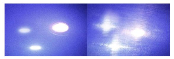
Haze is an important measure for highly polished metals and is often associated with polishing marks and machining direction.
