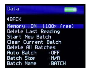
The Data & Batch Screen is similar in functionality to that of the menu screen but also allows the selection and setting of the Auto Batch size.
