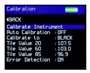
The Calibration Screen is used to setup the instrument calibration to the user's preference. Press the Up / Down buttons to navigates through the options, press the Enter button to select the option required.
