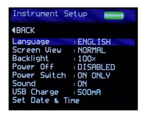
The Instrument Setup screen is used to configure the instruments basic operating environment to the user's preference. Press the Up / Down buttons to navigate through the options, press the Enter button to select the option required.
