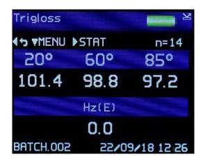
With ASTM E430 selected an (E) identifier will be displayed next to the Hz parameter. With ASTM D4039 selected a (D) identifier will be displayed next to the Hz parameter
