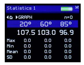
If the Pass / Fail feature is enabled, the colour of the angle header indicates if the last reading is within the user defined tolerances.
