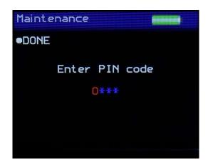
The Maintenance screen is used by Rhopoint Approved Service Centres. It is PIN locked to prevented unauthorised access.
