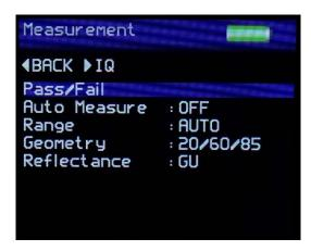
The Measurement Screen is used to configure the instruments measurement parameters to the user's preference. Press the Up / Down buttons to navigate through the options, press the Enter button to select the option required. Press the right button to enter the IQ Screen\*
