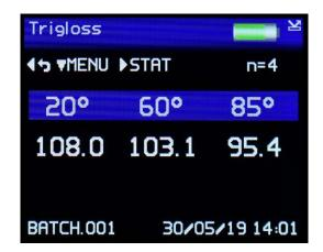
With the pass / fail feature enabled, the Novo-Gloss will compare each measurement angle to user defined tolerances. If the gloss reading is within specification, the angle header will be displayed in Green. If the reading falls outside the tolerances the header is marked in Red.
