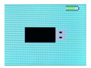
USB Remote Control - Allows control of the Novo-Gloss remotely by sending ASCII commands from a computer or PLC. In this mode the instrument displays "REMOTE CONTROL ACTIVE" on the main measurement screen.
