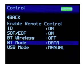
The Control Screen is used to configure the instruments Bluetooth parameters to the user's preference. Press the Up / Down buttons to navigate through the options, press the Enter button to select the option required.
