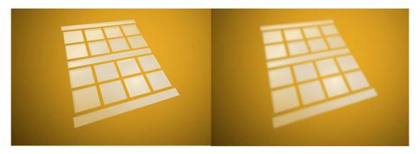
When viewing the reflection of a strong light source in a surface with high haze the image "blooms" and has a bright halo around it.
