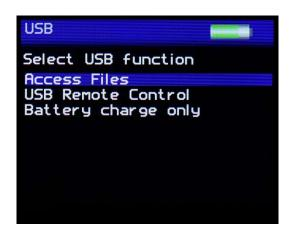
Access Files – Allows access to measurement and configuration files on the instrument. The instrument appears as a USB drive named NG-METER. When selected the display on the instrument shows a USB memory key as shown below –
