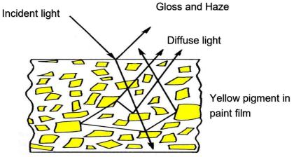
The Novo-Gloss compensates for reflection from within the coating for highly reflective pigments, metallic coatings and speciality pigments, allowing the haze of any painted surface to be measured.
