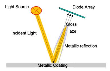
The Novo-Gloss captures compensation information from a region adjacent to the haze measurement angle, this means it can be used on metallic coatings which reflect light directionally
