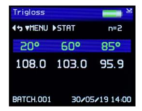
Press the Right button in the Home screen to access the gloss statistics screen for the current batch for all three angles. Measurements can be taken whilst in this screen and the statistics will be updated.
