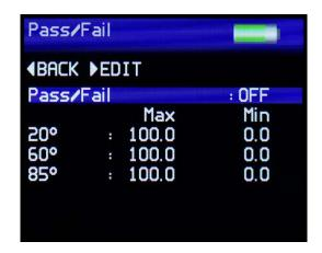
The Pass / Fail Setup screen is used to enable/disable on screen pass/fail indication and set measurement criteria.
