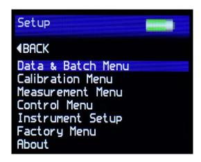
The Setup Screen is used to customise the instrument to the user's preference. Press the Up / Down buttons to navigate through the options, press the Enter button to select the option required.
