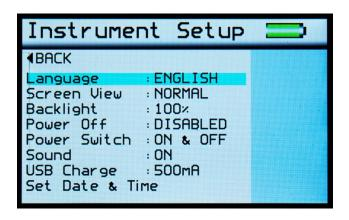
The Instrument Setup screen is used to configure the instruments basic operating environment to the user's preference. Pressing the Up and Down buttons navigates through the options, pressing the Enter button selects that option.
