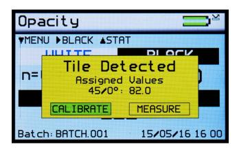
Two options are available: either to "Calibrate" the instrument on the calibration tile before making the measurement or to "Measure" without performing a calibration. Using the Left/ Right (3) and Enter (4) buttons on the keypad the required option can be selected.
