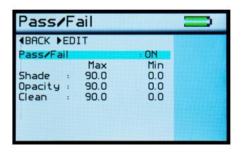
The Pass/Fail setup screen is used to enable/disable on-screen pass/fail indication and set min/max tolerancing.
