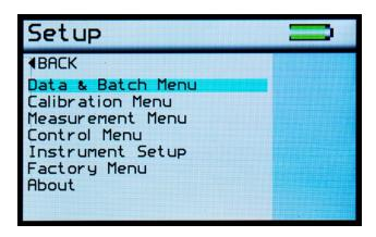
The Setup Screen is used to customise the instrument to the user's preference. Pressing the Up and Down buttons navigates through the options, pressing the Enter button selects that option.
