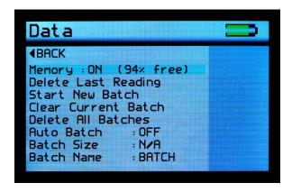
The Data Screen is similar in functionality to that of the menu screen but also allows the selection and setting of the Auto Batch size.
