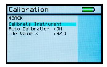
The Calibration Screen is used to setup the instrument calibration to the user's preference. Pressing the Up and Down buttons navigates through the options, pressing the Enter button selects that option.
