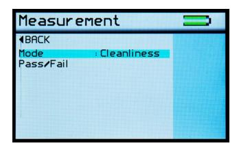
The Measurement Screen is used to configure the instruments measurement mode to the user's preference. Pressing the Up and Down buttons navigates through the options, pressing the Enter button selects that option.
