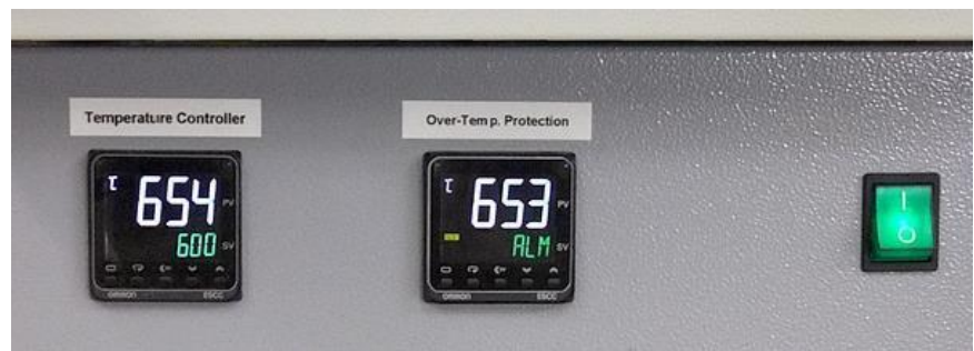
An example of the standard E5CC Temperature Controller and OTP 2 (Over-Temp. Protection). 'ALM' flashes on the display when over temperature.
