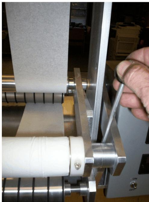
Figure 4: Lifter Block Handle
