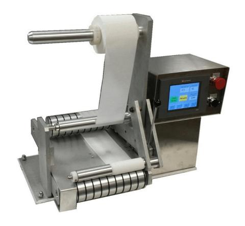
The RLC -13 provides accurate and reliable test data pertaining to the Roll lengths of consumer tissue and paper rolls.
