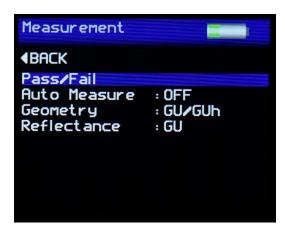
The Measurement Screen is used to configure the instrument's measurement parameters to the user's preference. Press the Up / Down buttons to navigate through the options, press the Enter button to select the option required.
