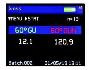
Press the Right button to access the statistics screen for the current batch. Measurements can be taken whilst in this screen and the statistics will be updated.
