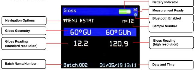
In this mode, measurements can be made by simply pressing any of the measurement buttons.
