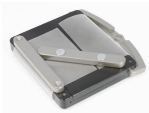
\* The sled has been calibrated to 200g including the magnet bars. If for any reason the magnet bars cannot be used to secure the sample use tape and then place the magnet bars on top.
