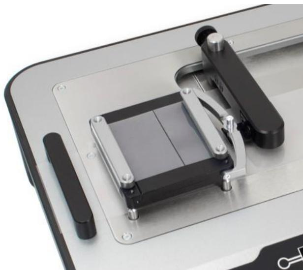
When in the home position menu press the
