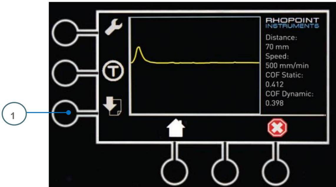
Once the export results button has been pressed the instrument will beep once to indicate a button press and again to indicate the export is complete. The USB stick can then be removed from the instrument and plugged into a PC device.
