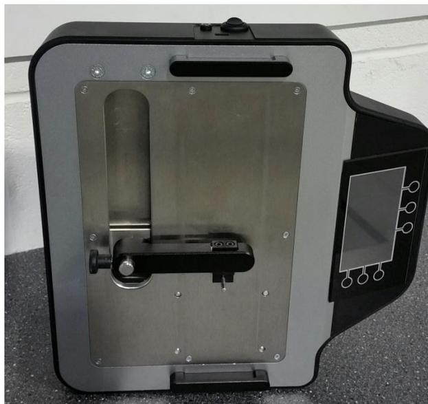
On the live load cell reading note the value shown. This is the mass of the load cell and sled coupling.
