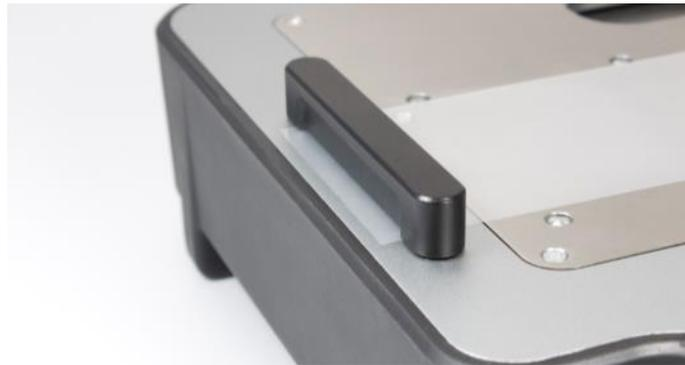
The sample size for the sled should be 63.5mm square. When measuring flexible samples the size can be 63.5x148mm and wrapped around the sled. The foam pad on the bottom will ensure a 63.5mm square contact area.
