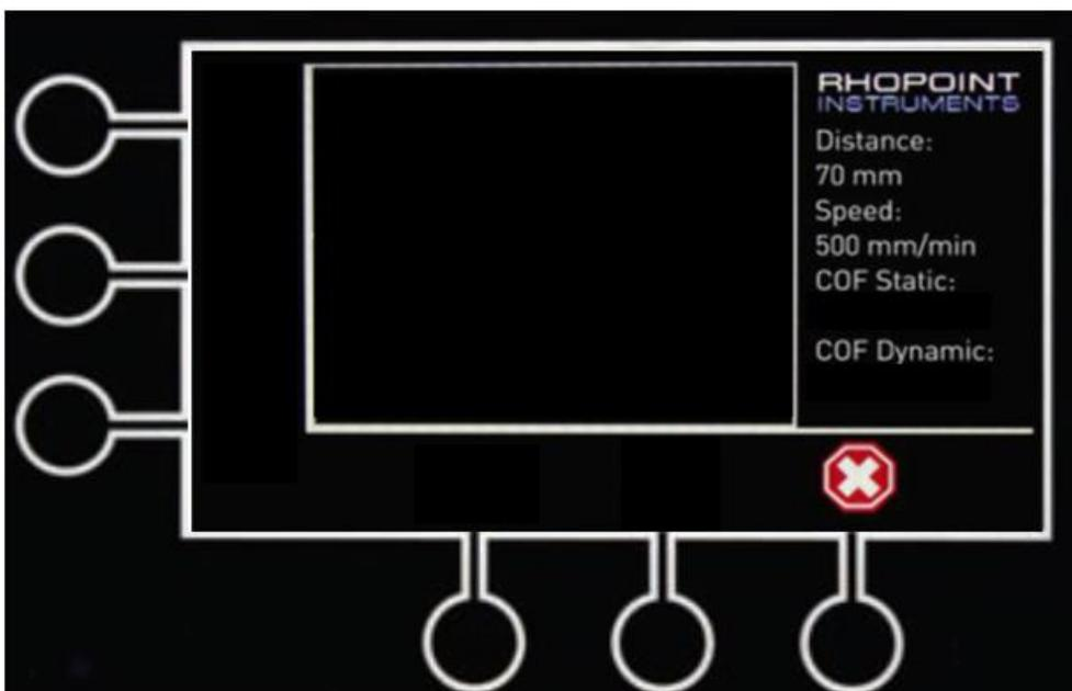
During the test a live reading from the load cell is shown on the graph. When the test has finished the graph will re-scale to maximize the graph display. The COF Static and COF Dynamic will be displayed bottom right of the screen.
