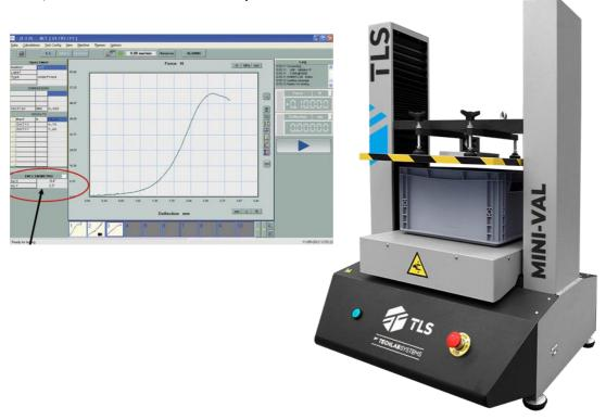
The Testing Software allows testing of Compression at Break, Compression at Constant Load and Cyclic Compression on Packaging and Packaging of Corrugated and Compact Cardboard, Plastic, Metal ...
