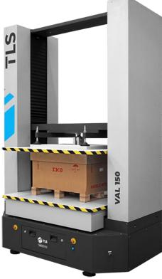
The Testing Software allows testing of Compression at Break, Compression at Constant Load and Cyclic Compression on Packaging and Packaging of Corrugated and Compact Cardboard, Plastic, Metal ...
