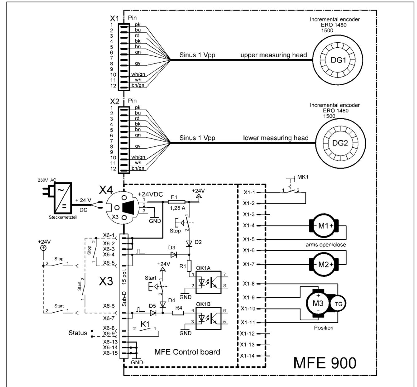
Picture 2: MFE 900 - Connection diagram
