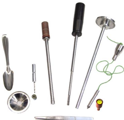
**Spatula** and pellet feeding **funnel**, Tungsten Carbide  $\varnothing$  2,095 mm **capillary die**, Capillary die **cleaning tool**, **Piston**, Cylinder **cleaning tool**, **Extrusion tool**, **Plumb line**, **Bubble level** and **Tweezers**.
