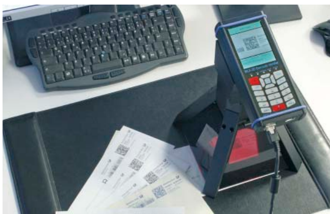
Verifying DataMatrix codes on mailing bags
