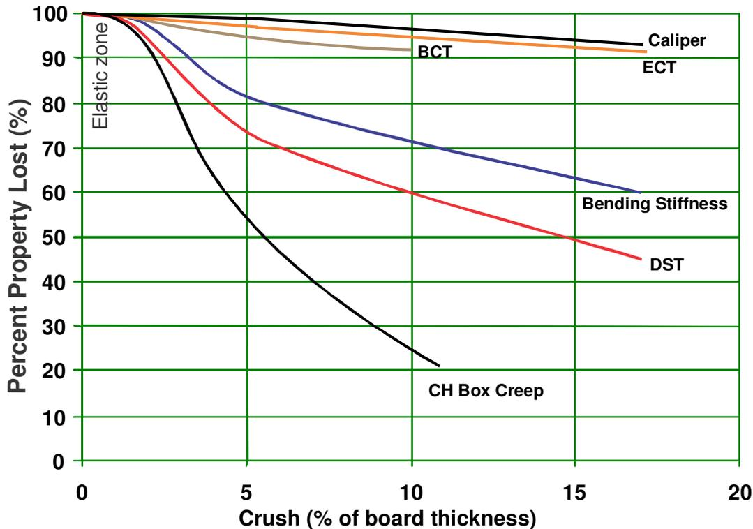
At 10% crush the Caliper is effected by about 3.5%, the ECT by 5%, the BCT by 8% the Bending Stiffness by 28%, the MD Torsional Stiffness by 40% and the Cyclic Humidity Box Compression Creep (CHBCC) by 75%. The BCT data finished at 10% crush but we believe that the line may trend more steeply down after about 12% crush.
