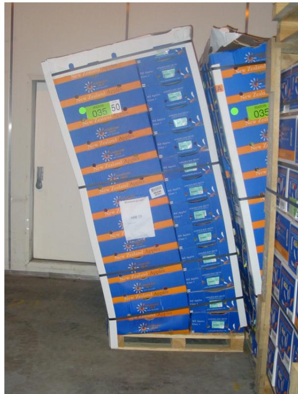
**Figure 1:** Collapsing stacks in high humidity storage environment.
