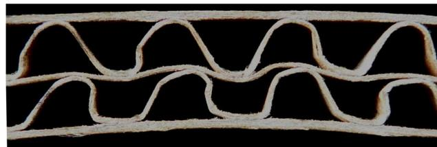
**Figure 3:** MD Torsional stiffness fails then bending stiffness fails.
