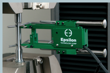
Model 3542 with 25 mm gauge length
