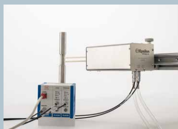
Model 7650 extensometer with Model DT6229 two-channel signal conditioner
