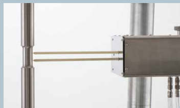
Model 7650 extensometer with 12.5 mm gauge length
