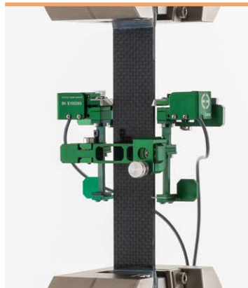
Model 3442AVG-050M-025M-ST with 50 mm gauge length and +2.5 mm/-1.0 mm measuring range
