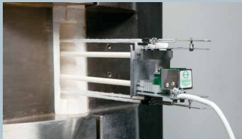
Self-supporting Model 3448 with clamshell-type materials testing furnace
