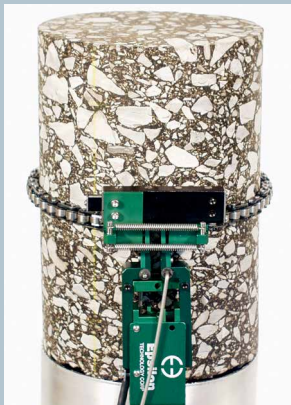
Model 3544-0400 with 1.25 inch to 4 inch diameter range
