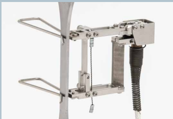
Model 7642-050M-125M extensometer
