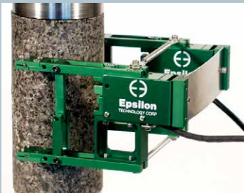
Model 3542RA1 extensometer with 50 mm gauge length
