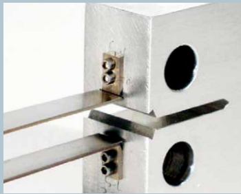
Model 3541 attached to bolt-on knife edges
