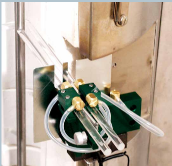
Model 3580 mounted to split furnace
