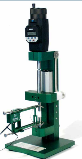
Model 3590 calibrator with Model 3542 axial extensometer
