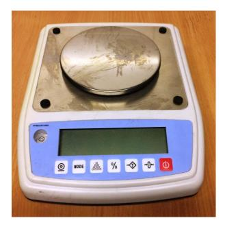
Powered by mains or internal rechargeable battery (50 hrs) - charger supplied Backlit LCD display with 16.5 mm high digits 14 weighing units
