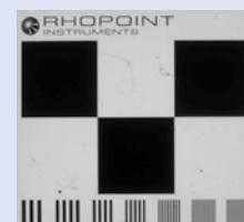
Image 1: Pristine film, 1mm air gap, measured with Rhopoint ID
