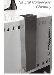
consider some fumes may escape around the door or if it is opened while hot. If the chimney is no longer needed, it can be blocked with suitable high temperature insulation wool (a small amount is supplied).
