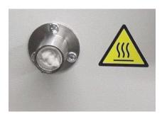
\*Thermocouples and metal objects must be suitably earthed and should be fitted by a suitably qualified person. Precautions must be taken to prevent contact with the exposed electric heating elements.
