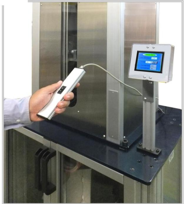
**NOTE:** We can build the impact resistance test equipment according to **ASTM D 2444** with drop height of the striker impact of **3 m** (please consult).
