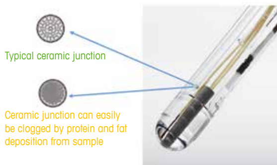
Figure 2: Sample impact on a conventional pH sensor having a ceramic junction
