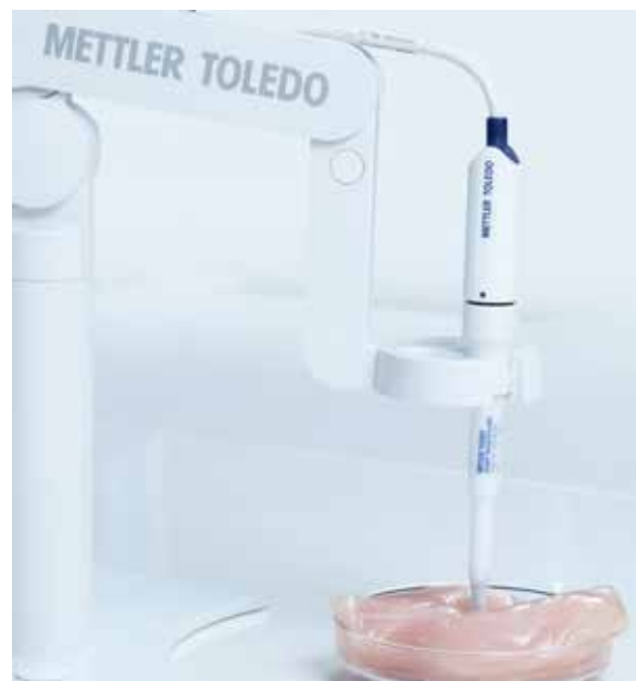
Figure 3: Measuring pH of poultry sample using InLab Solids Pro-ISM pH sensor
