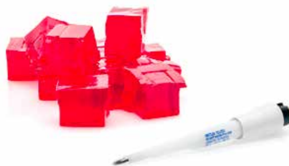
Figure 3: InLab Solids Pro-ISM sensor to measure the pH of jelly samples
