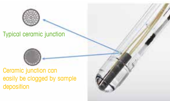
Figure 1 : Sample impact on a conventional pH sensor having a ceramic junction
