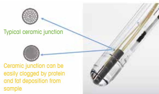
Figure 2: Sample impact on a conventional pH sensor having a ceramic junction
