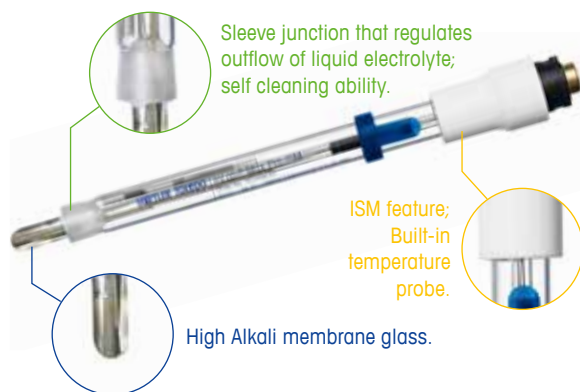
Figure 2: InLab Max Pro-ISM pH sensor.
