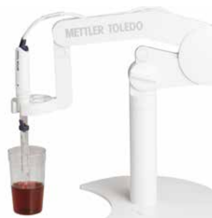
Figure 3: Measuring a wine sample using InLab Max Pro-ISM sensor.
