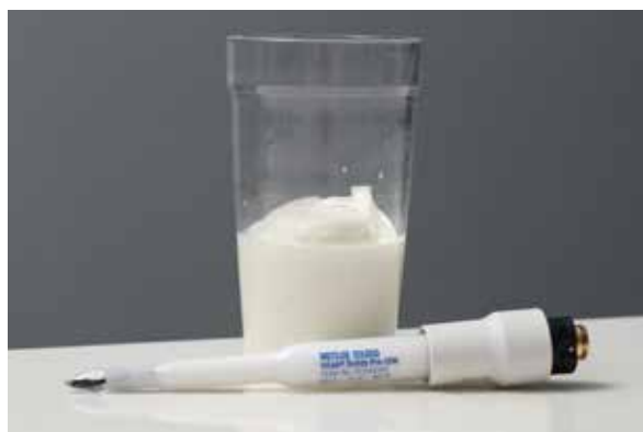
Figure 2: Measurement of whipped cream sample using InLab Solids Pro-ISM pH sensor
