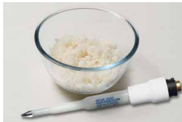
Figure 2: Measurement of cooked rice using InLab Solids Pro-ISM pH sensor
