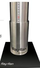
usually compressed to lessen the bulk, a measure of their density under a small compression load is very useful. For this test a measuring cylinder of 1000cm<sup>3</sup> is supplied along with a scaled weight plunger with 1mm graduations on the outside. Lead shot is used to increase the plunger weight to 2300g to compress the material under test.
