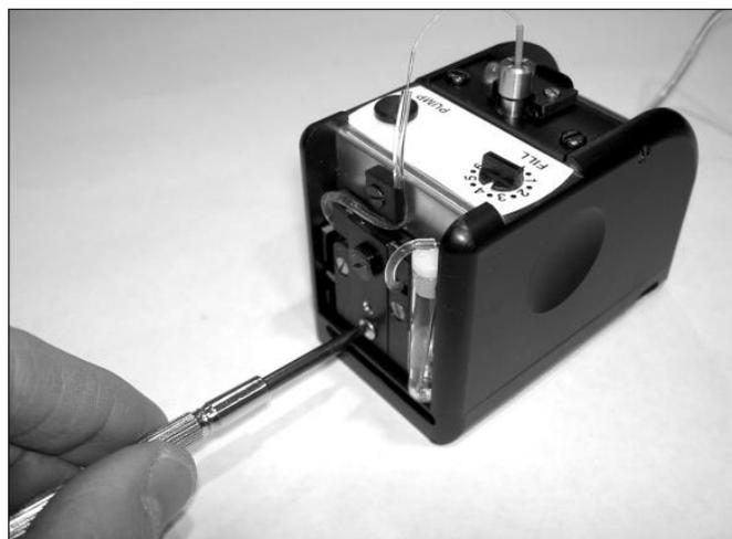
*Tighten the pump lid screw*
