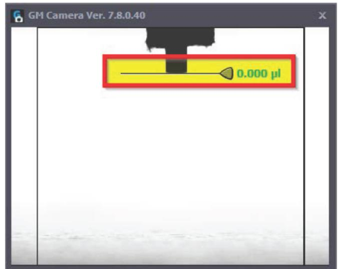
described as "wetting hysteresis", is characterised by the highest ("advancing") and lowest ("receding") contact angles. This test is based on a reversible pump flow. The optional PG Dosing Unit is a programmable dispenser suitable for this task, but any stand-alone pump with reversible flow can be used for the test. With a little practice it is even possible to use a regular handheld syringe to run this test manually.
