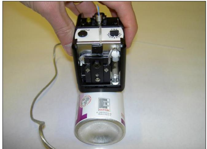
Testing curved surfaces perpendicular to the object axis
