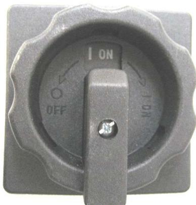
Figure 20: Power switch (K) of the voltage and frequency changer in position "ON"
