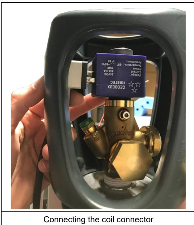
Connecting the coil connector
