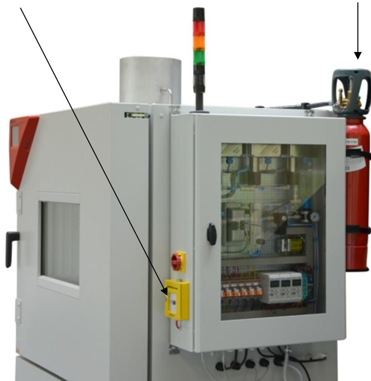
Figure 12: Location of the devices for the CO<sub>2</sub> fire suppression device
