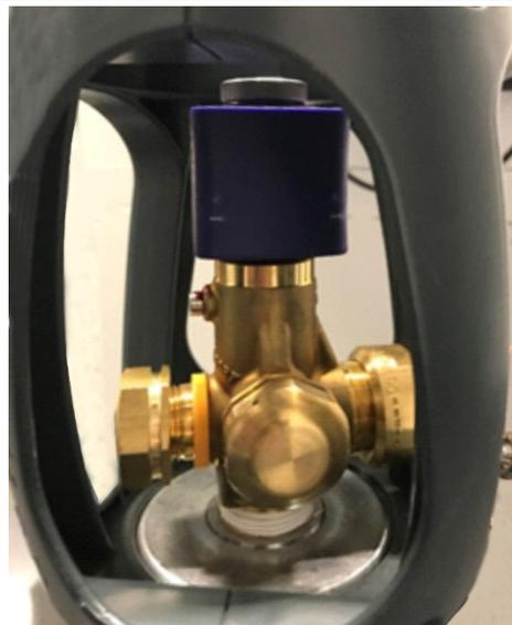
Valve with mounted solenoid coil
