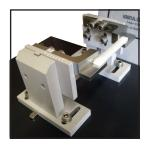
the subsequent impact strength calculated. Complies to International Test Standards ISO 179, ASTM D256, ASTM D6110, DIN 53453, DIN 53753, and BS 7413. Impact hammer energies are available from 0.5J up to 50J.
