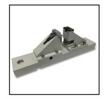
supported as a horizontal beam similar to Charpy tests conditions and complies to International Test Standards ISO 7628 and ISO 9854. Sample diameter dimensions up to 25mm (0.98in) can be tested with hammer energies of 7.5 - 15J (5.6 - 11.1 ft-lbs) or 50J (36.9 ft-lbs), as defined in the ISO standards.
