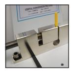
or Un-notched specimens can be tested using the Izod method. Complies to International Test Standards ASTM D256, ASTM D4812 and ISO 180. Impact hammer energies are available from 0.5J up to 25J.
