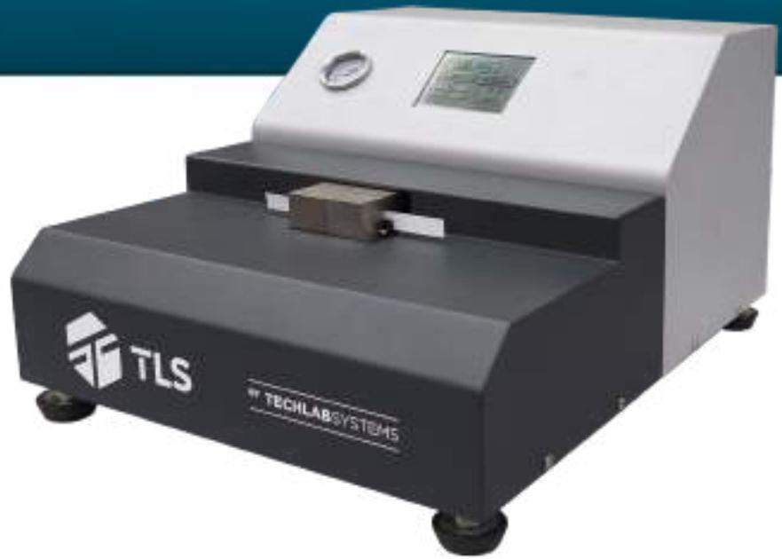
This testing equipment is used to measure the compressive strength of paper and cardboard samples by the SCT method (0.7mm short distance compression between jaws). The test is performed using a 15 mm wide paper or cardboard specimen and it is compressed until failure occurs.
